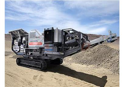
2. Ship-shaped steel chassis. It is of high intensity, low on ground pressure etc. And it is easy to be transported on different terrains like mountain and marsh.
